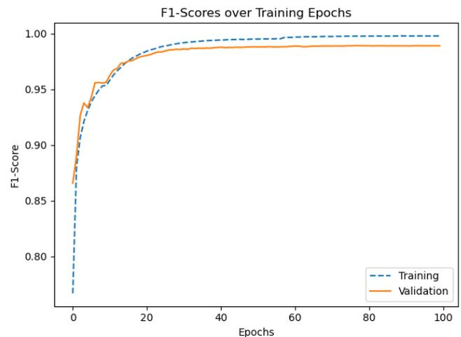
**Figure 4: The progress of the score for the final training for 100 epochs. The progress shows an asymptotic behaviour after around about 40 epochs.**
