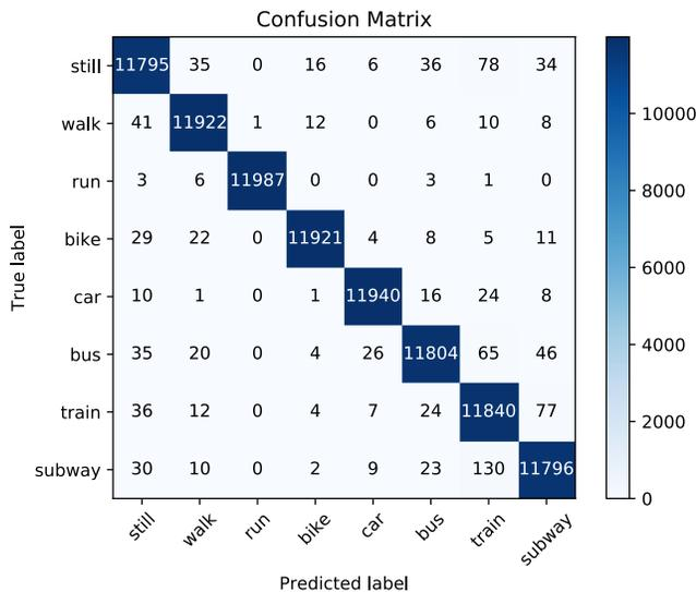
**Figure 6: The Confusion Matrix for the internal test set. The classes with the most false classifications *still* and *subway*. The classes with the best true classifications are *run* and *walk*.**
