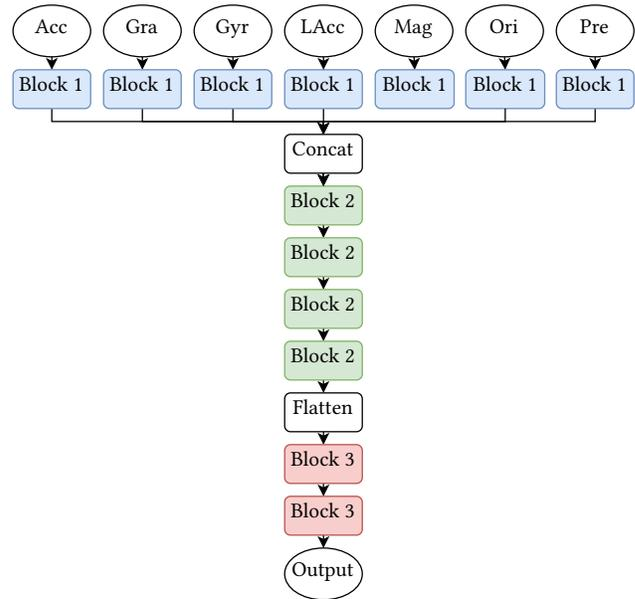
**Figure 2: The architecture of the model. Each sensor modality had its own input and the intermediate features were fused in the concatenation layer in the second dimension.**
