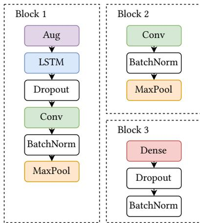
**Figure 3: A detailed view of the three different blocks of layers used in our architecture.**
