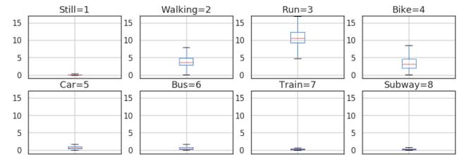
Figure 2: Boxplots of the standard deviation of acceleration for all classes.
