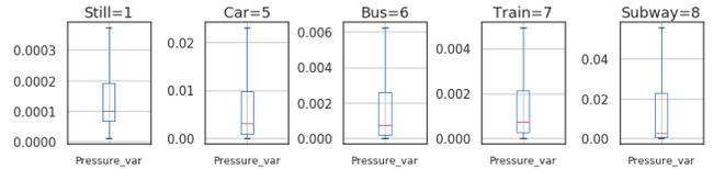
**Figure 5: Boxplots of the variance of pressure with labels of still, car, bus, train and subway.**
