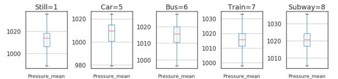
**Figure 6: Boxplots of the average of pressure with labels of still, car, bus, train and subway.**
