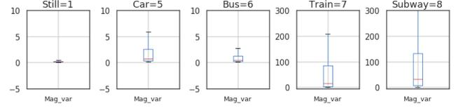
**Figure 4: Boxplots of the variance of magnetic field with labels of still, car, bus, train and subway.**
