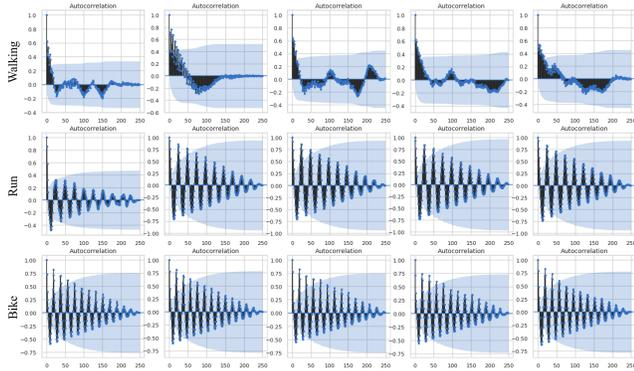
**Figure 3: Auto-correlation of  $LA_v$  while walking, running and biking.**
